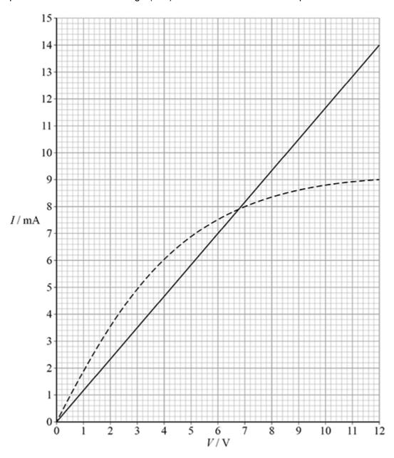
The two components are connected in parallel with a 12 V battery that has negligible internal resistance.
