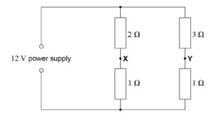
What is the reading on a voltmeter connected between points **X** and **Y**?
