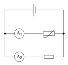
The cell has a constant electromotive force and negligible internal resistance. Readings from the two ammeters are taken.
