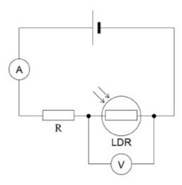
Which row shows how the readings on the ammeter and the voltmeter change when the light intensity incident on the LDR is increased?
