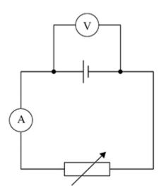
When the resistance of the variable resistor is 10  $\Omega$  the voltmeter reads 10 V and the ammeter reads 1.0 A.
