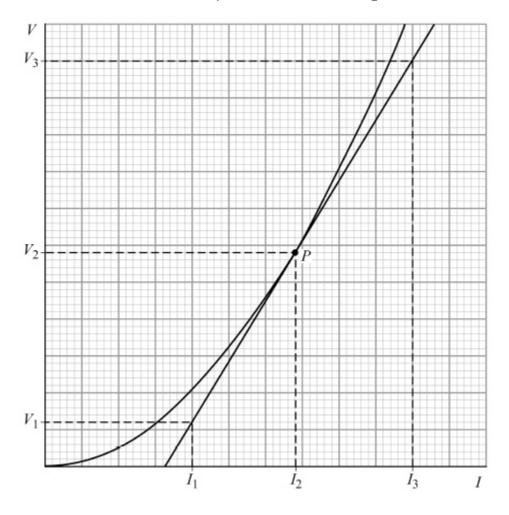
What is the resistance of the electrical component when the current in the component is  $I_2$ ?
